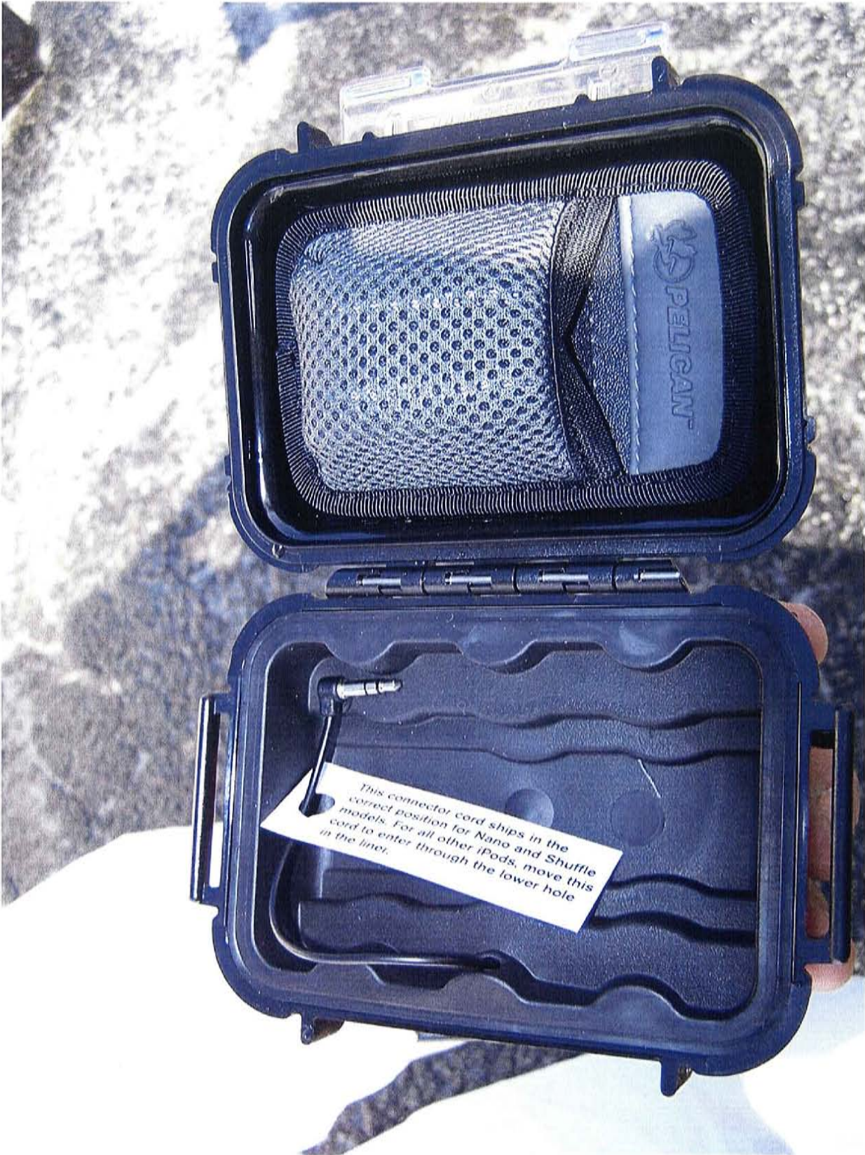
Photograph 6 Water Ingress Post Test
